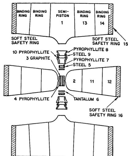
Fig. 1 “Exploded” View of the Belt High Pressure, High Temperature Apparatus
