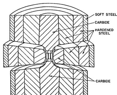
**Fig. 2 "Closed" View of the Belt High Pressure, High Temperature Apparatus**
